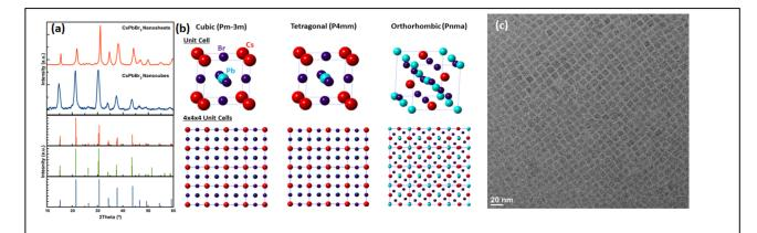
**Figure 1**. (a) XRD patterns for CsPbBr<sub>3</sub> nanocubes and nanosheets, (b) atomic arrangements for 3 crystal phases and (c) typical TEM image of CsPbBr<sub>3</sub> nanocubes.
