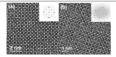
**Figure 2.** HRTEM images of two types of CsPbBr<sub>3</sub> nano-crystals: (a) nanocubes and (b) nanosheets. Inserted are Fourier Transform Patterns indicating that nano-cubes (a) have a cubic structure at room temperature while nano-sheets (b) have an orthorhombic structure.
