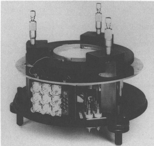
Figure 2: The CasFPer servo-stabilised FP, Mark I
