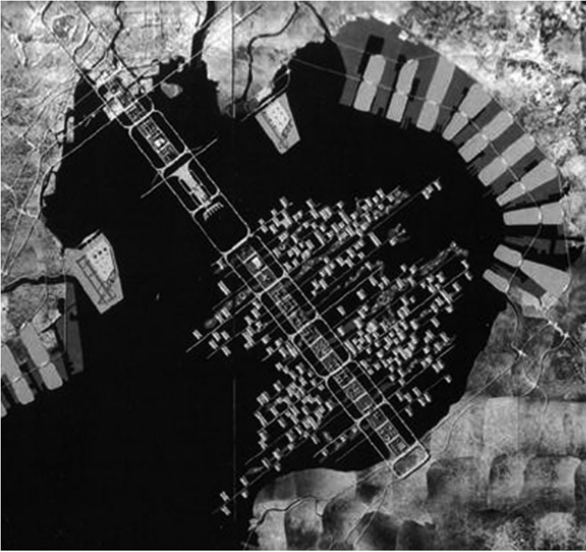
Figure 1. Bird's-eye view of Tange Lab's 'Plan for Tokyo 1960': the cycles of the Civic Axis lineally cross the Bay from Tokyo to Chiba Prefecture, with residential areas perpendicular and parallel to them. Source: Tange et al., Tōkyō keikaku 1960 , p. 30. Photo taken by © Akio Kawasumi, courtesy of Tange Associates (Tokyo) and TKTA.
