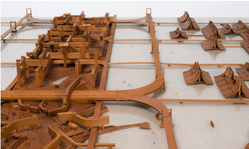
Figure 3. View of one loop, with office buildings suspended between huge cores located inside it, and a residential area with elevated A-frame structures perpendicular and parallel to it. Source: Kenzō Tange, Tokyo Bay Model , KTA_D001-002_023 (seq. 23), TKTA, https://iif.harvard.edu/manifests/view/drs:45367752123i , [accessed 16 June 2021]. Courtesy of TKTA.
