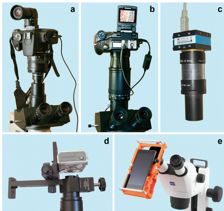
Figure 3: Examples of camera-microscope setups. (a) Digital SLR camera fitted with a suitable lens adapted to a trinocular photo-tube with a photo eyepiece 10 \times . (b) Digital bridge camera with an integrated zoom lens mounted with a vario (zoom) photo ocular 5 \times to 12.5 \times . (c) Special microscope camera mounted with a photo eyepiece 10 \times . (d) Compact digital camera mounted with a monocular tube. (e) Smartphone-adaptor (UNIKOP, manufactured by Immunocons Co., Germany) mounted with a stereo microscope. This adapter consists of a variable holder so that smartphones of different sizes can be used.
