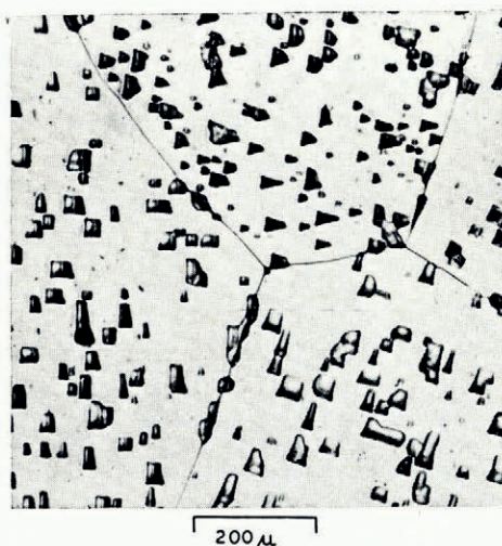
Fig. 7. Grain boundaries forming two tri-crystal joints on a formvar replica of the ice surface. Etch figures are also shown
