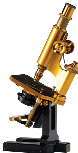
Figure 6: Stand with micrometer movement and tilt from 1882, from the collection of Timo Mappes. Photograph taken by Manfred Stich.
