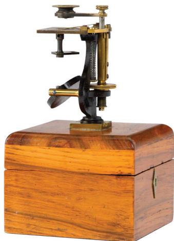
Figure 3: Dissection microscope with dovetail mount, produced in this form until 1848, from the collection of Timo Mappes. Photograph taken by Manfred Stich.
