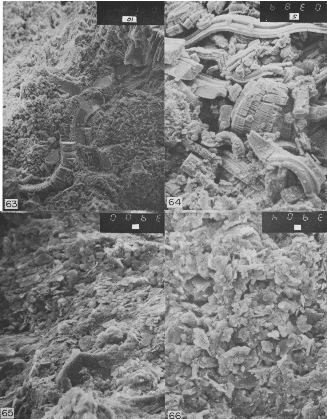
Figure 63. Large S-shaped book (vermiform) of kaolinite, Hodges mine, Georgia Kaolin Co., 0187, 750 \times .
