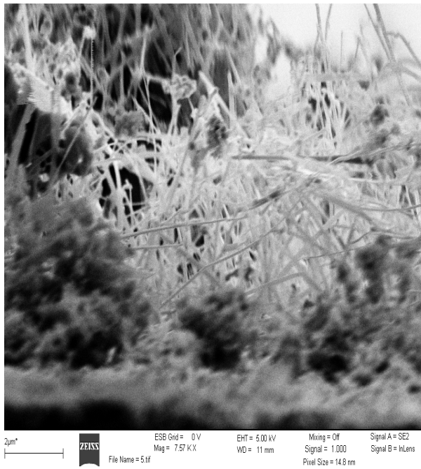
FIG 1. SEM side view of the CdSSe nanowires. The scale marker is 2 μm long.
