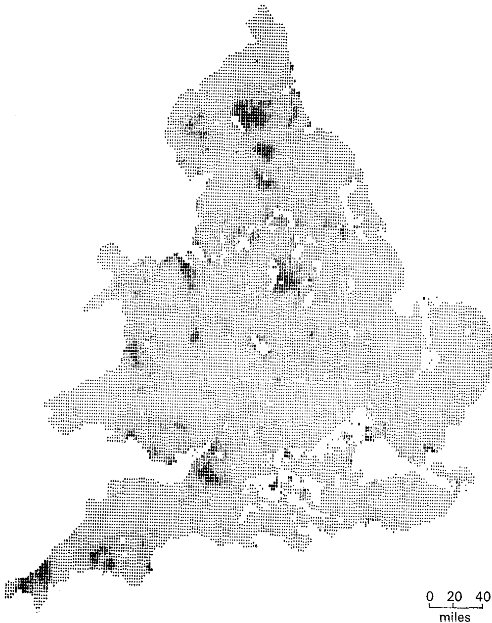
Fig. 1. Provisional map showing the distribution of lead in stream sediment in England and Wales, based on a modification of the grey-scale mapping programme described by Howarth (1971). [□], Less than 40 \mu\text{g Pb/g} ; [▤], 40–80 \mu\text{g Pb/g} ; [▥], 80–160 \mu\text{g Pb/g} ; [▧], 160–320 \mu\text{g Pb/g} ; [▨], >320 \mu\text{g Pb/g} .
