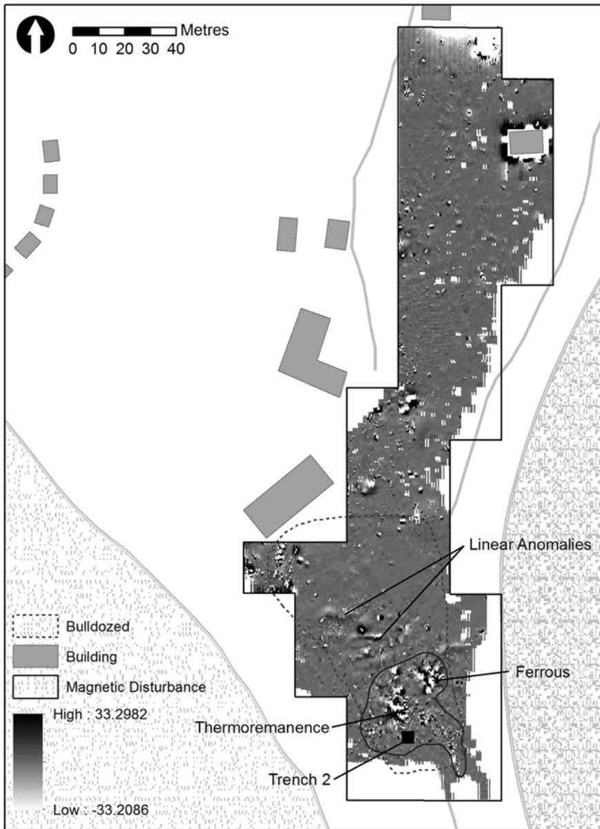
Figure 4. Magnetometry results from the survey of area A, showing the location of anomalies, ferrous materials, thermoremanence and the placement of trench 2.
