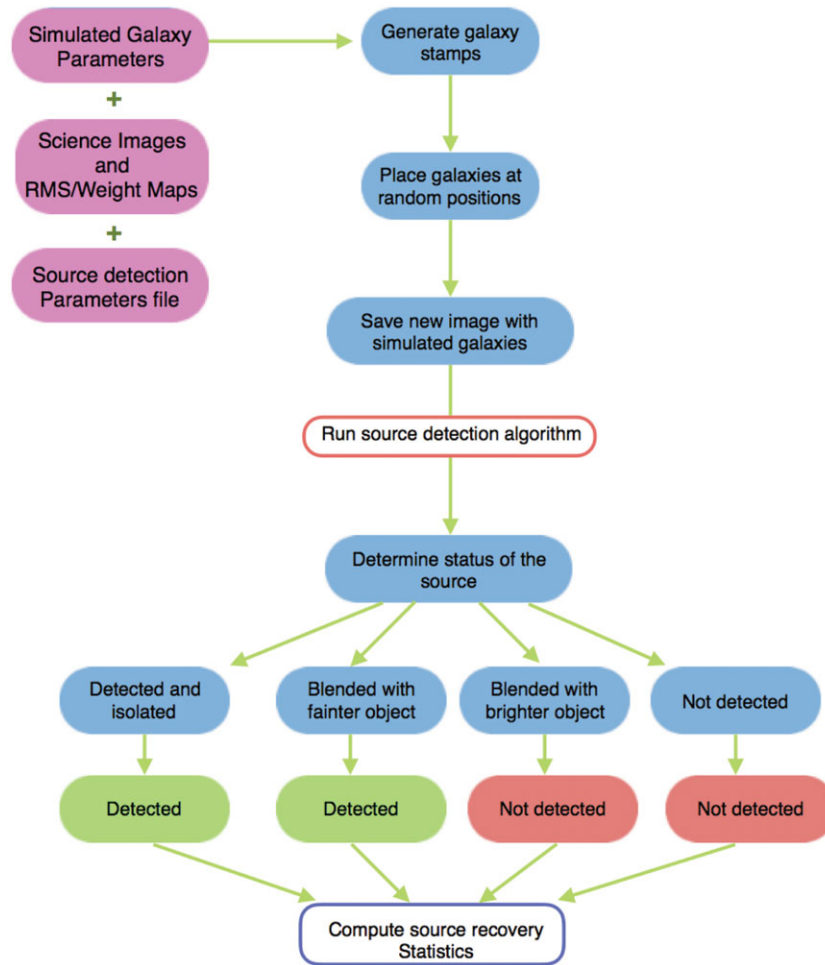
Figure 1. Logic diagram of GLACiAR's code structure. User-defined parameters and a science image (with its associated RMS map) are taken as input, with the code then generating simulated galaxy stamps, which are added to the science image at random positions, sampled from a uniform distribution. A detection algorithm is run on these images, and its output is used to determine statistics on source recovery.
