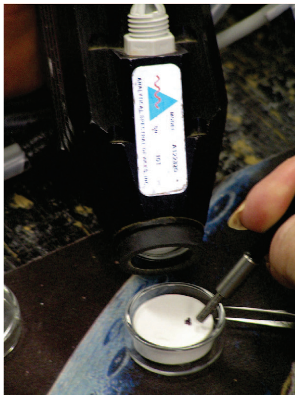
Figure 2. Fiber optic cable used to capture directly a VNIR-SWIR spectrum from a small discrete garnet grain.
