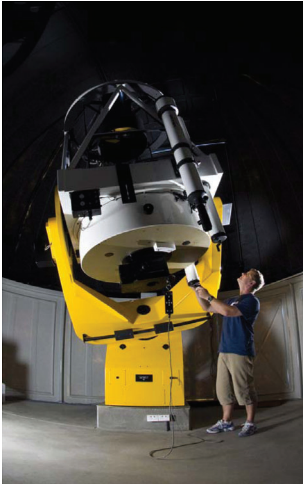
Figure 1 Zadko Telescope: a new 1 m f/4 Cassegrain reflector, located 67 km north of Perth. Built by DFM Engineering, Inc., and donated to UWA by resource company Claire Energy. It was opened by Australia's Chief Scientist on 1 April 2009.
