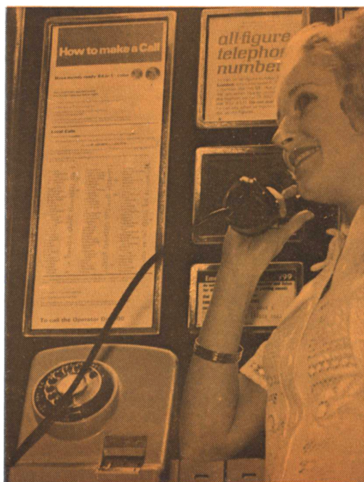
Casing of an S.T.D. coin box made at H.D.A.'s pressure die foundry.
