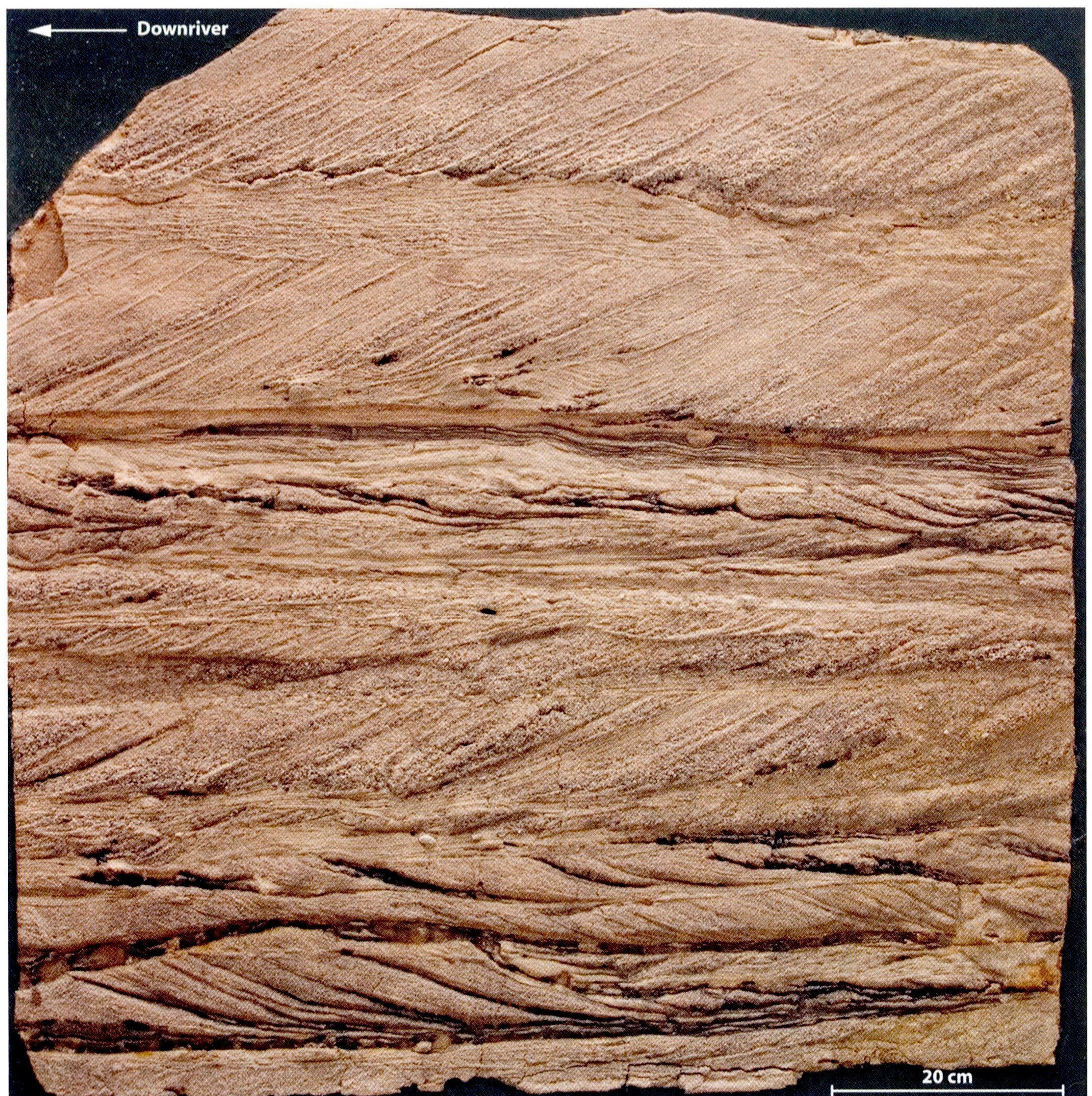
Fig. 12. Two successive cycles of flood directed cross-stratification followed by downriver fluvial X bedding. Note the presence of clay drapes in the flood-directed sets (formed by migration of ripples and dunes to the left). The sets generated by the upriver flow have a fine sand texture, whereas the fluvial X-beds consist of coarse sand. This demonstrates the much stronger downriver flow (Hambach exposure).
