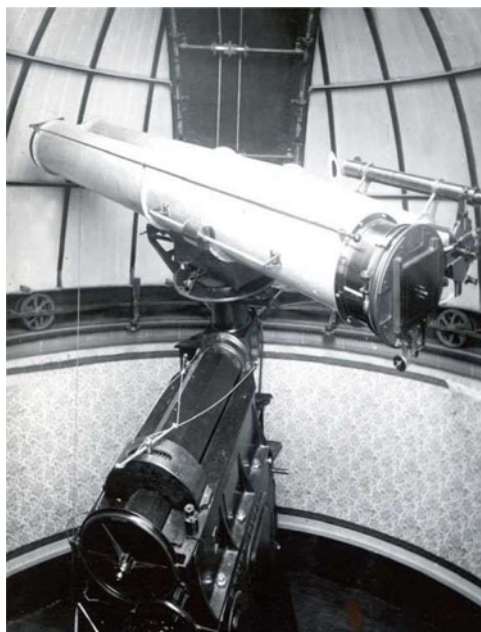
Figure 6. Observatory of Tacubaya astrographic telescope, manufactured by H. Grubb (Institute of Astronomy of the National Autonomous University of Mexico).
