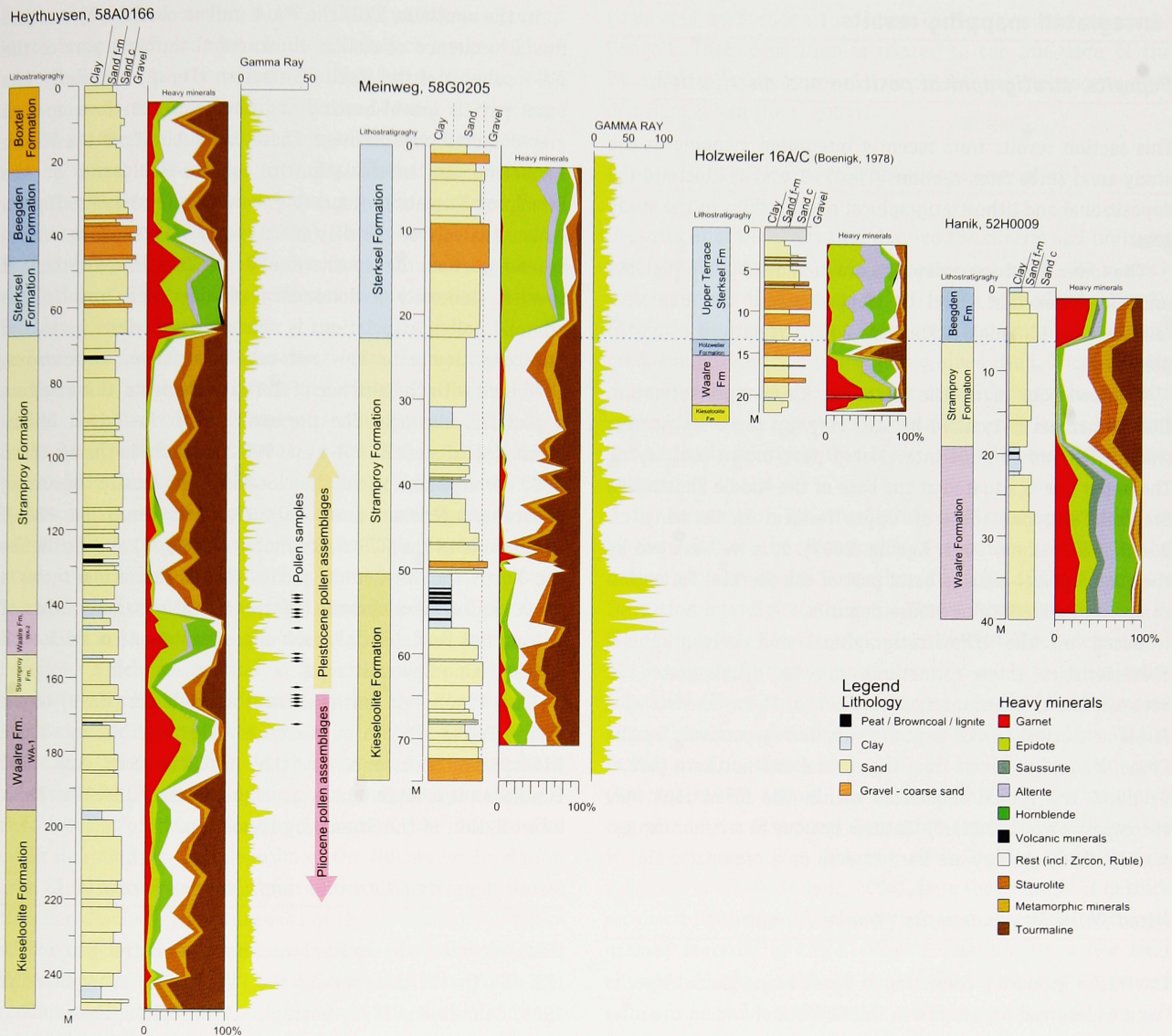
Fig. 6. Lithology, gamma-ray curves, heavy minerals and lithostratigraphy from 4 key sites in the study area (localities indicated in Fig. 1). Note that the Stramproy Formation may be underlain by different lithostratigraphical units of various ages and exhibits a highly variable thickness.
