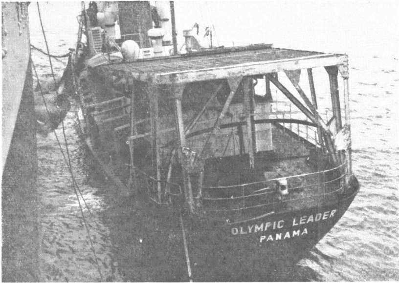
Fig 1 A small platform on the "Olympic Leader" as arranged for the Hiller 360
