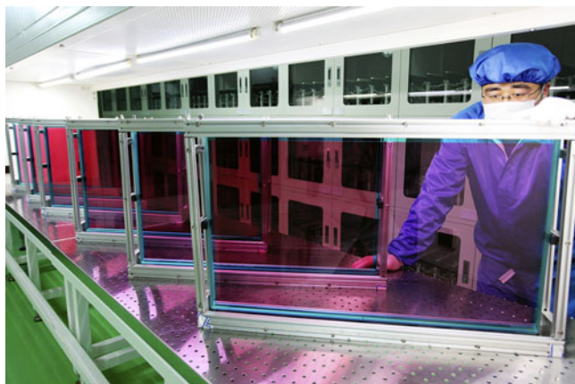
Figure 6. 400 mm aperture N31 glass slabs before installation.
