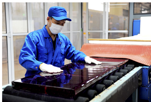
Figure 2. Large size N31 glass running from the annealing Lehr of a continuous melting line.
