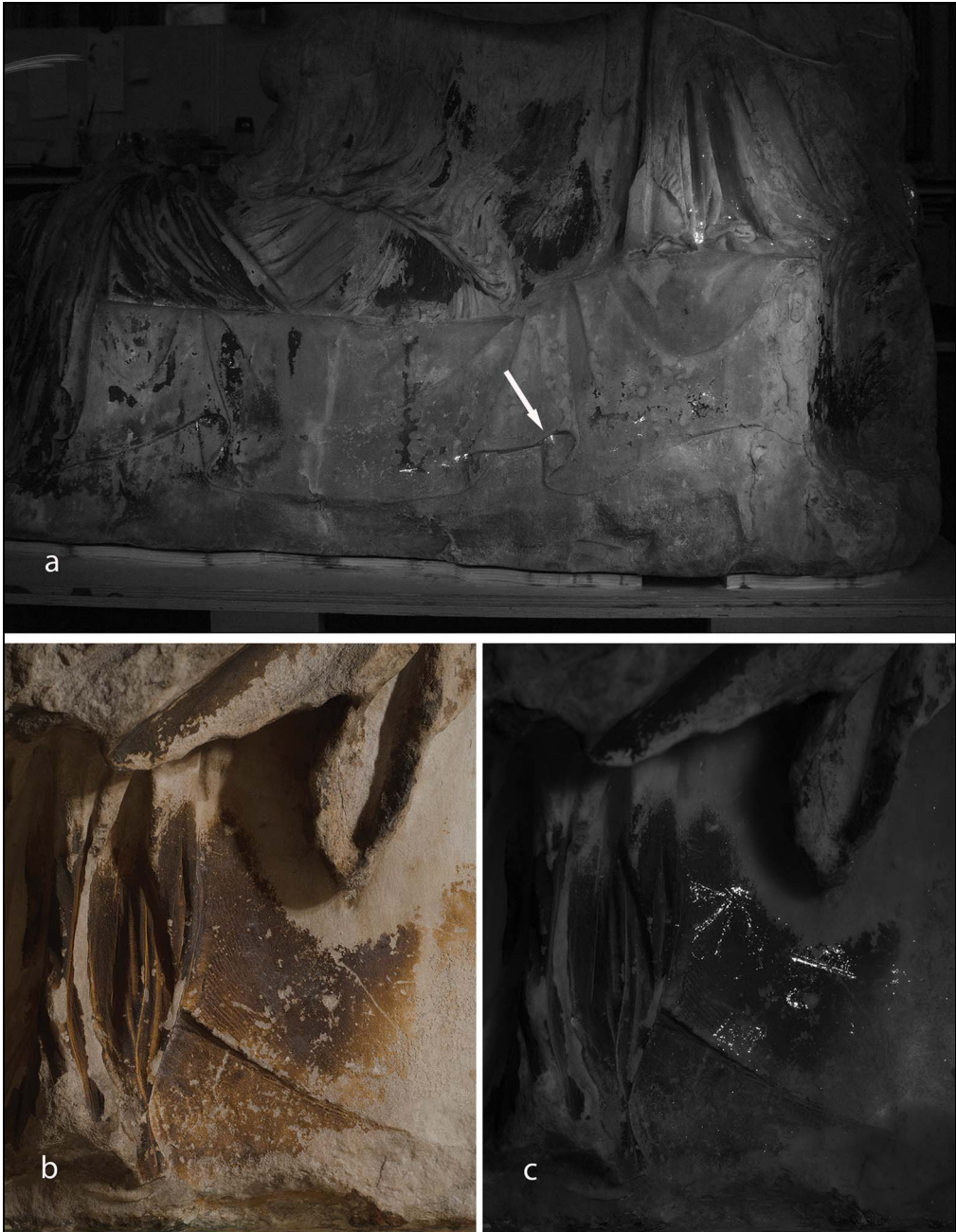
Figure 7. Figure EP L and M: VIL image of a) the back and b) visible and c) VIL image of a detail of the front by L's feet. The white arrow in (a) shows the sample location for Raman and SEM-EDX analysis (figure by Giovanni Verri) © Trustees of the British Museum.
