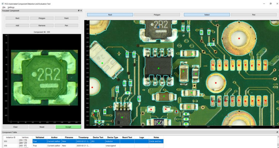
Figure 1. Overview of the annotation tool. Main UI components include an overview of the whole image, a zoomed-in view of the currently selected component, and a table of current component properties.
