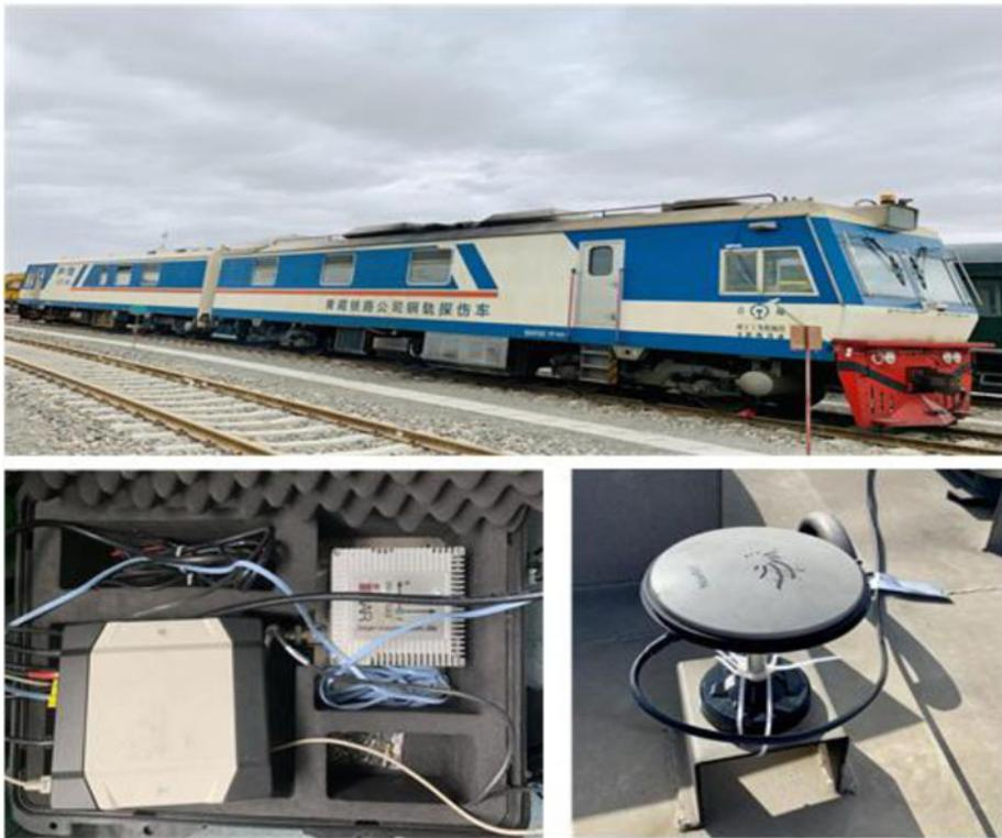
**Figure 5.** Testing train and experimental device.
