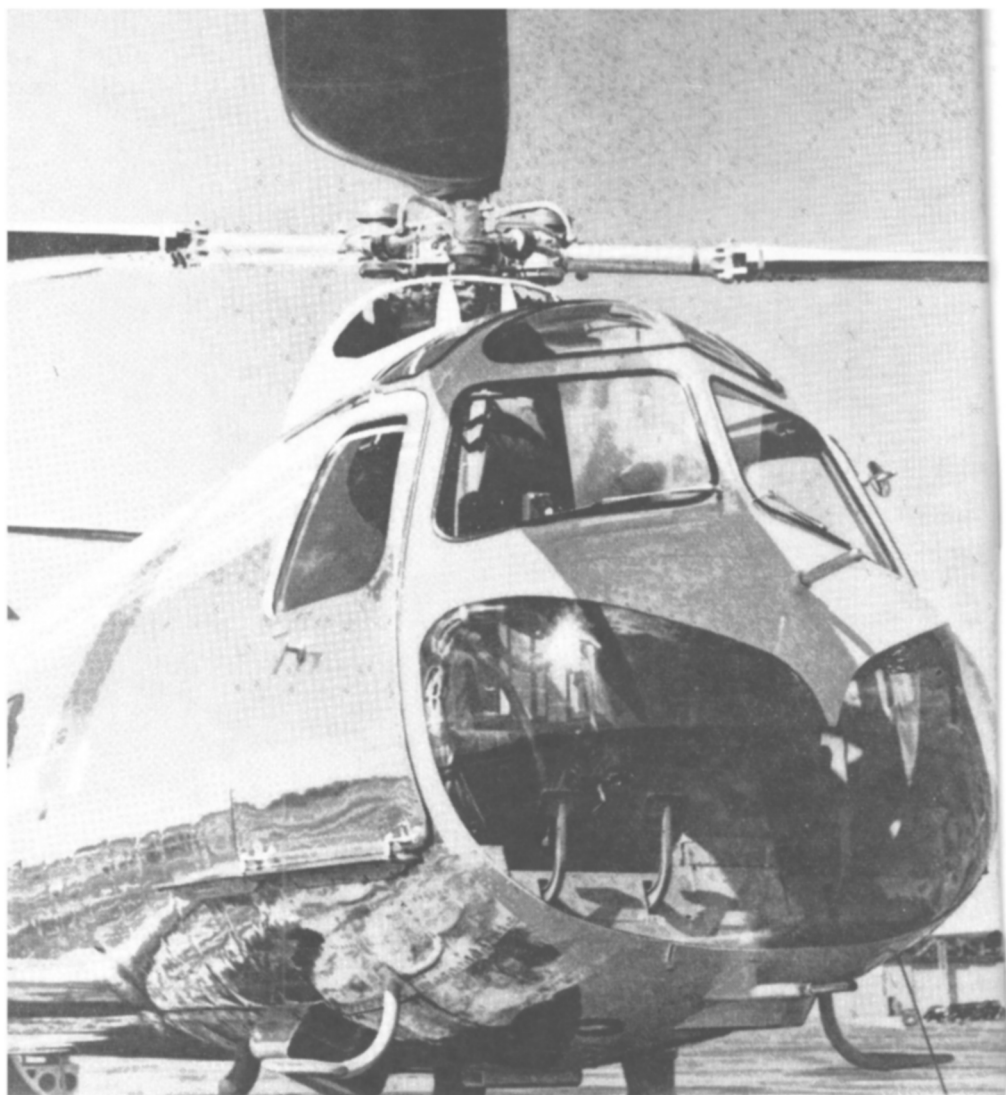
A BRISTOL 173 TANDEM ROTOR HELICOPTER POWERED BY TWO ALVIS LEONIDES ENGINES
