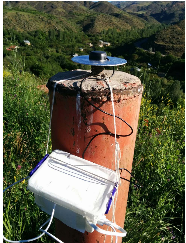
FIGURE 2. Reach circuit board and antenna, used as the base station and placed on the concrete surveying point.
