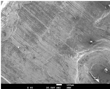
Figure 2. SEM image of the gold solidus showing striations due to die striking.
