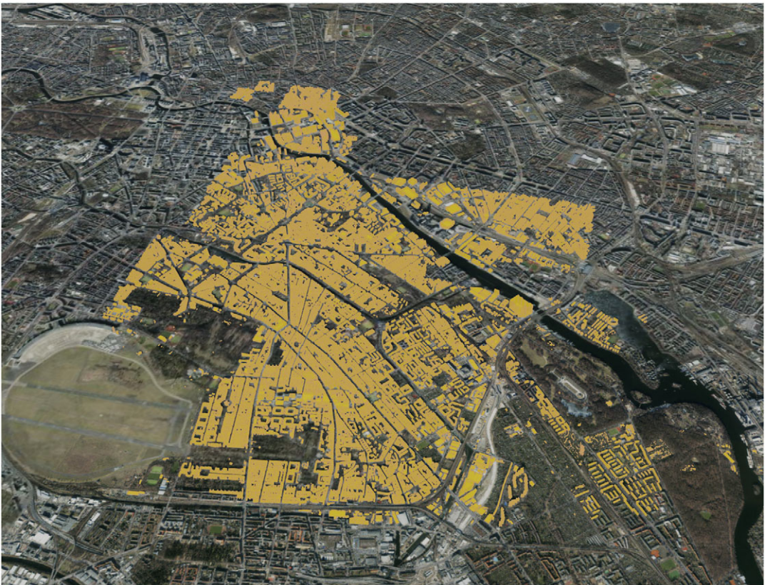
Figure 4. Visualization of Berlin on the dynamic knowledge graph architecture of the Cities Knowledge Graph, part of the World Avatar Project. KML tiles for visualization are dynamically loaded based on the current scope. Typical problems found in traditional GIS systems that relate to model updates have been solved. Partial model updates are possible and, thanks to the design of the City Export Agent, reflecting changes on the user interface is not a problem anymore.
