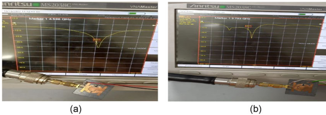
Figure 9. (a) S_{11} on VNA for case 1 and (b) S_{11} on VNA for case 2.
