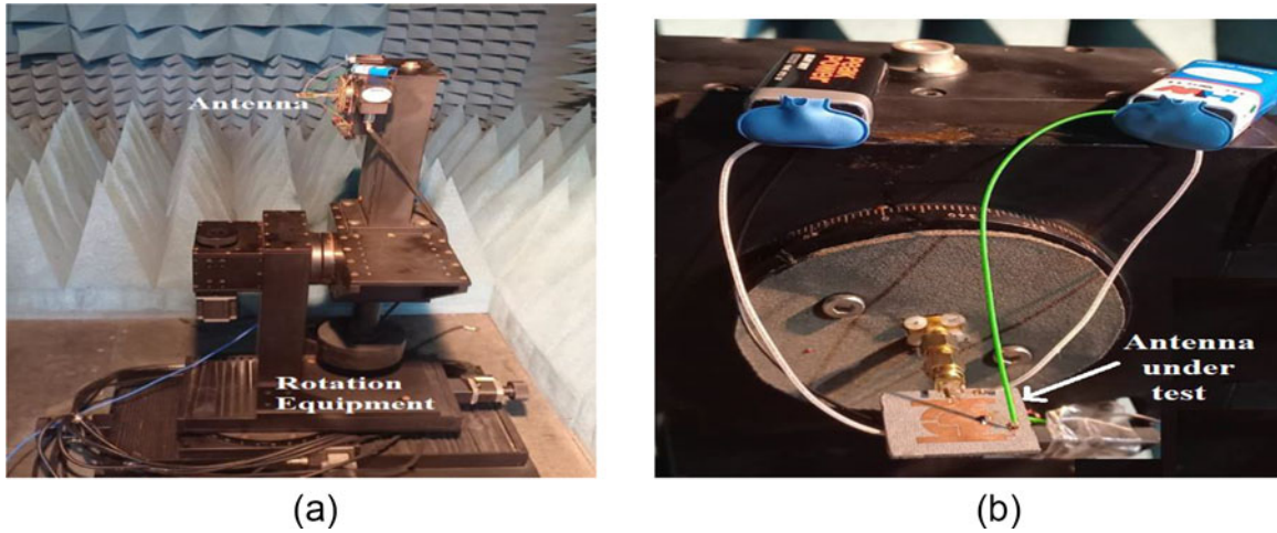
Figure 12. Inside the Anechoic chamber: (a) mechanical rotation system and (b) antenna under test.
