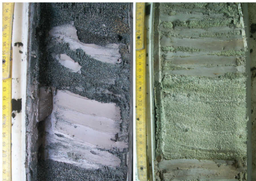
Figure 2. (left) Glauconitic sands of the Diest Formation intercalated with thin, irregular clay layers. (right) Slightly glauconitic sands of the Kasterlee Formation with thin clay intercalations.
