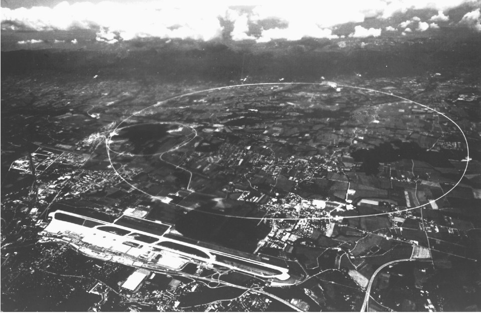
Fig. 1.3. An aerial view of CERN-Geneva, showing the underground LEP ring, 27 km in circumference, where also the LHC (large hadron collider) will run soon. In order to see the real size of the ring, one can see Geneva airport in the front part of the photo (ref. CERN X 973-1-87).
