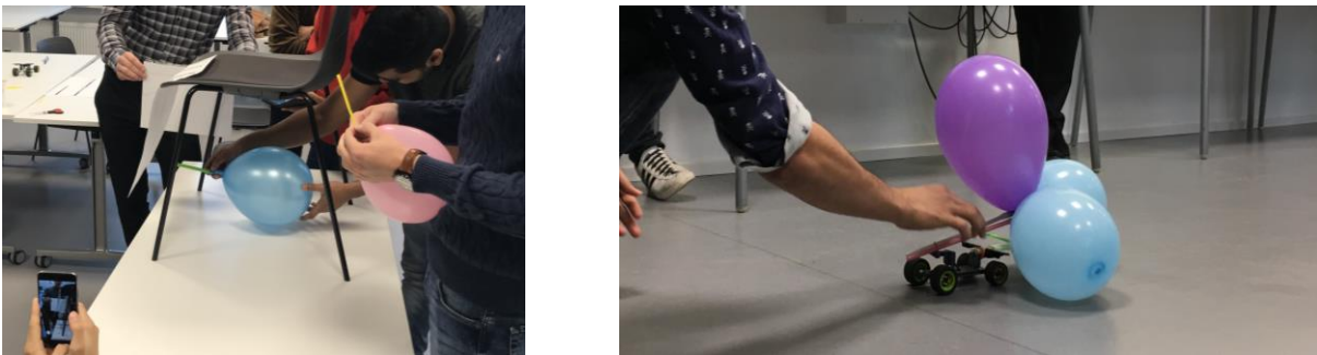
Figure 5. (a) innovative test-rig from one of the teams for measuring the properties of different balloon settings during the research phase, (b) one of the solutions during the race/evaluation phase, consisting of three balloons each connected to a straw and mounted on a vehicle.
