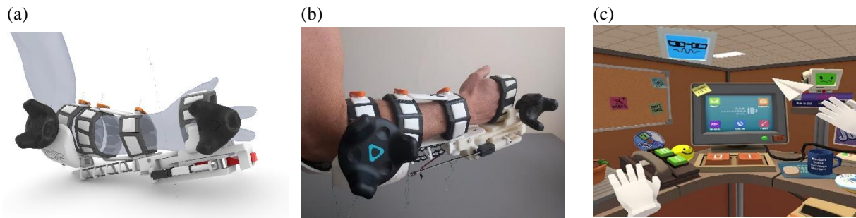
Figure 4. (a) The established model in CAD; (b) Creation of the initial prototype; (c) “Job Simulator” setting integrated within the VR environment for use during therapy
