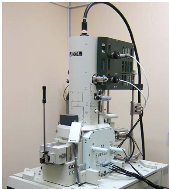
Figure1. This figure shows JSM-7100F, equipped with the Gatan 3View 2XP.
