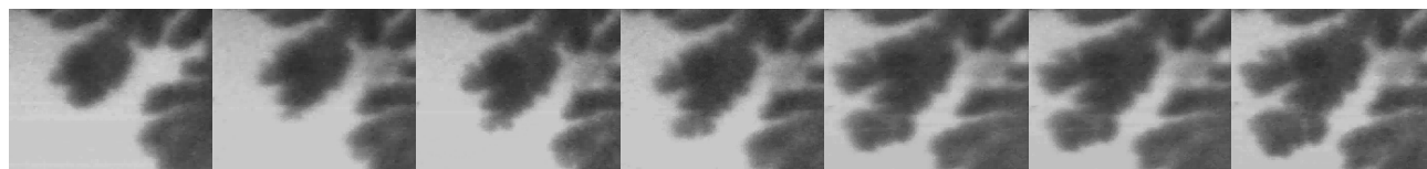
FIG. 2. Series of bright field, energy filtered images extracted from a video recorded in situ showing the growth of dendritic arms of copper from the edge of a polycrystalline Au electrode. The electrolyte was 0.1M \text{CuSO}_4/\text{H}_2\text{SO}_4 and growth conditions were galvanostatic with 40 \text{mAcm}^{-2} (1 mA total current). Images are shown at 8 second intervals. The field of view is 6.25 \mu\text{m} .
