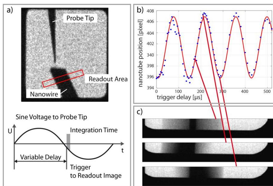
**Figure 2.** Overview image of nanowire and probe tip position in a). A sine voltage was applied to the probe tip inducing oscillations in the nanowire. The shadow of the vibrating nanowire was imaged with an integration time of 25  $\mu\text{s}$ . The center of gravity of these images was calculated and plotted against the trigger delay in b). Single images of the readout area are shown in c) for three different delays.
