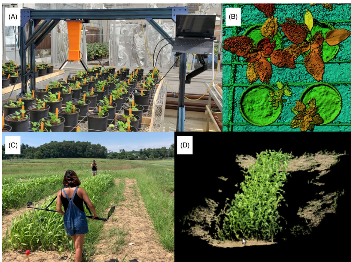
Figure 1. (A) BenchBot autonomous high-throughput imaging system, (B) example imagery from BenchBot after automated segmentation of weeds from background objects, (C) testing of the handheld version of the Weeds3D system at the Beltsville Agricultural Research Center, and (D) example 3D reconstruction of plant biomass from the Weeds3D systems.
