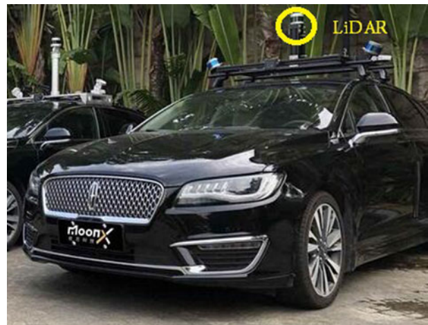
Fig. 5. A picture of the LiDAR and the corresponding passenger car used to capture the proposed dataset.
