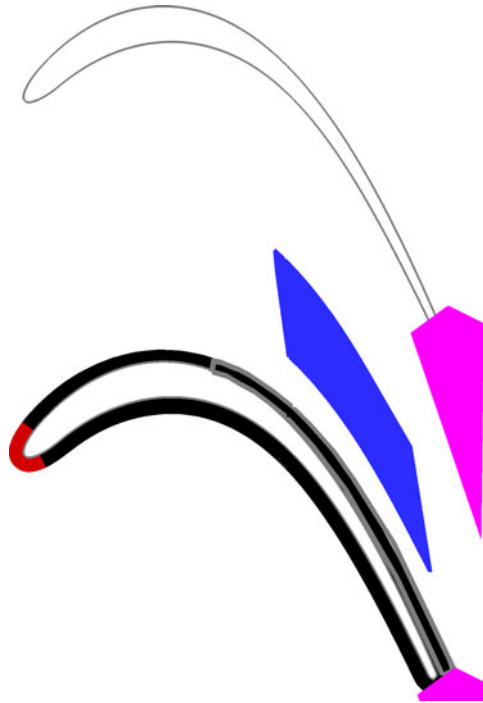
Figure 3. Domains used for extraction of data sets for computation of temporal/spanwise basis for extended POD projection: red, leading edge; black, boundary layer; blue, rear part of the passage; pink, wake region; grey, rear part of the suction side of the boundary layer.
