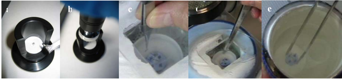
Figure 1: Minimizing contamination during specimen preparation: (a) loading the filter paper disk and protective backer using the loading jig, (b) attaching the filter paper and protective backer onto a blotter, (c) transferring the frozen hydrated grid within the cryogenic atmosphere of the liquid nitrogen workstation, (d, e) frozen hydrated grids within the transfer pot are submerged in liquid nitrogen as they are removed to a storage dewar.
