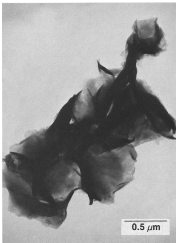
Figure 7. Transmission electron images of foliated aggregate of smectite flakes formed from Mg 2+ -bearing gel on reacting at 300°C and 500 bars for 35 days.
