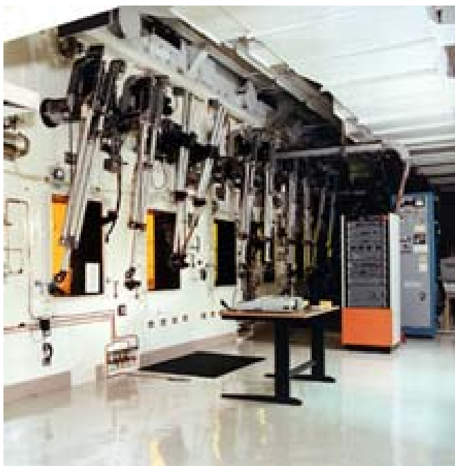
Figure 1: Irradiated Materials Examination and Testing (IMET) hot cell facility.
