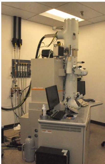
Figure 3: JEOL 2100F TEM/STEM instrument. Equipped with EDS and EELS+EFTEM, this tool is now available for irradiated materials and fuels work in LAMDA.
