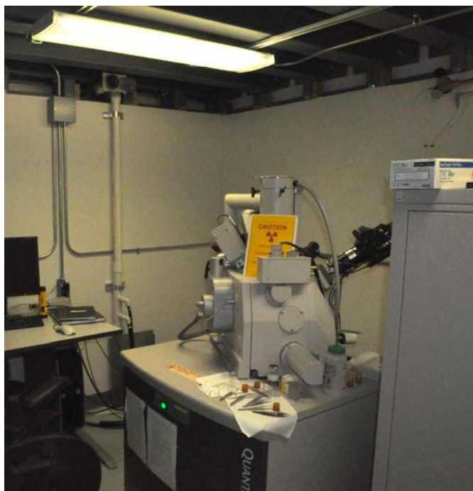
Figure 2: FEI Quanta DualBeam FIB-SEM system. A second operator control station, separated from the instrument by a lead wall, protects the operator from strongly gamma-emitting specimens.
