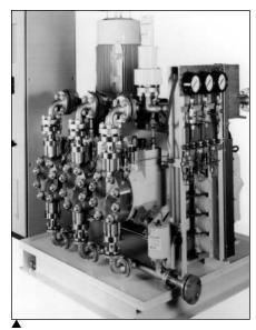
Diaphragm Metering Pumps for CO<sub>2</sub> Applications: LEWAtriplex<sup>™</sup> Monoblock metering pumps from American LEWA handle liquid CO<sub>2</sub> at up to 10,000 psi. The pumps feature a leak-free sealless diaphragm with positive displacement and low pump-head volume. The pumps can be equipped with cooling jackets and special materials to meet user requirements. Contact: sales@amlewa.com; www.amlewa.com.
