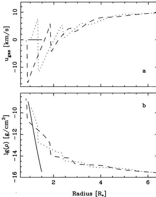
Figure 3. Radial structure of a dynamic model at different phases (0.50: dashed, minimum light; 1.00: dotted, maximum light) and of the corresponding hydrostatic initial model (full line); flow velocity (a) and gas density (b) as a function of the radius (given in units of the radius of the hydrostatic initial model). The wind of this O-rich model is driven by radiation pressure on molecules (no dust formation included). Model P7OU4 of Höfner et al. (1998).
