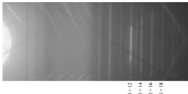
Fig. 2. CBED pattern with the reflections 0012 – 0021 satisfying the Bragg condition.
