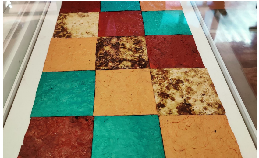
Figure 8. Tapestry of mycelium leather pieces measuring 12 cm × 12 cm treated with acrylic paint.
