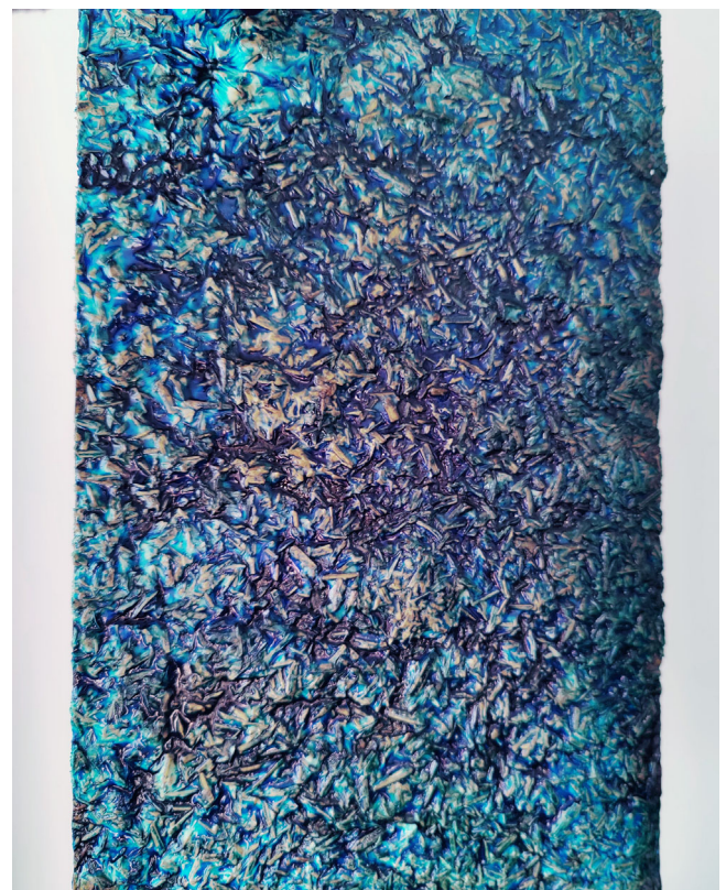
Figure 9. Mycelium leather samples measuring 30 cm × 48 cm grown using Ecovative living material, treated with blue algae solution using a spray-on application.
