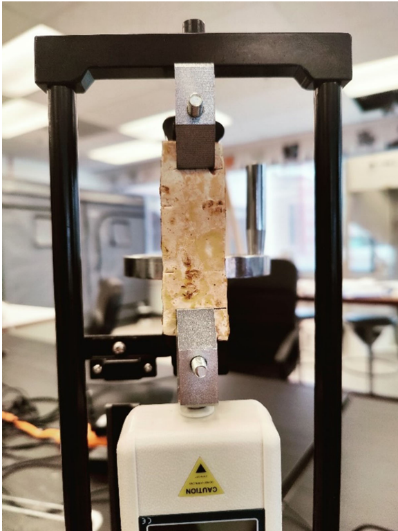
Figure 2. Tensile testing of mycelium samples using Mxmoonfree Digital Force Gauge 500N.
