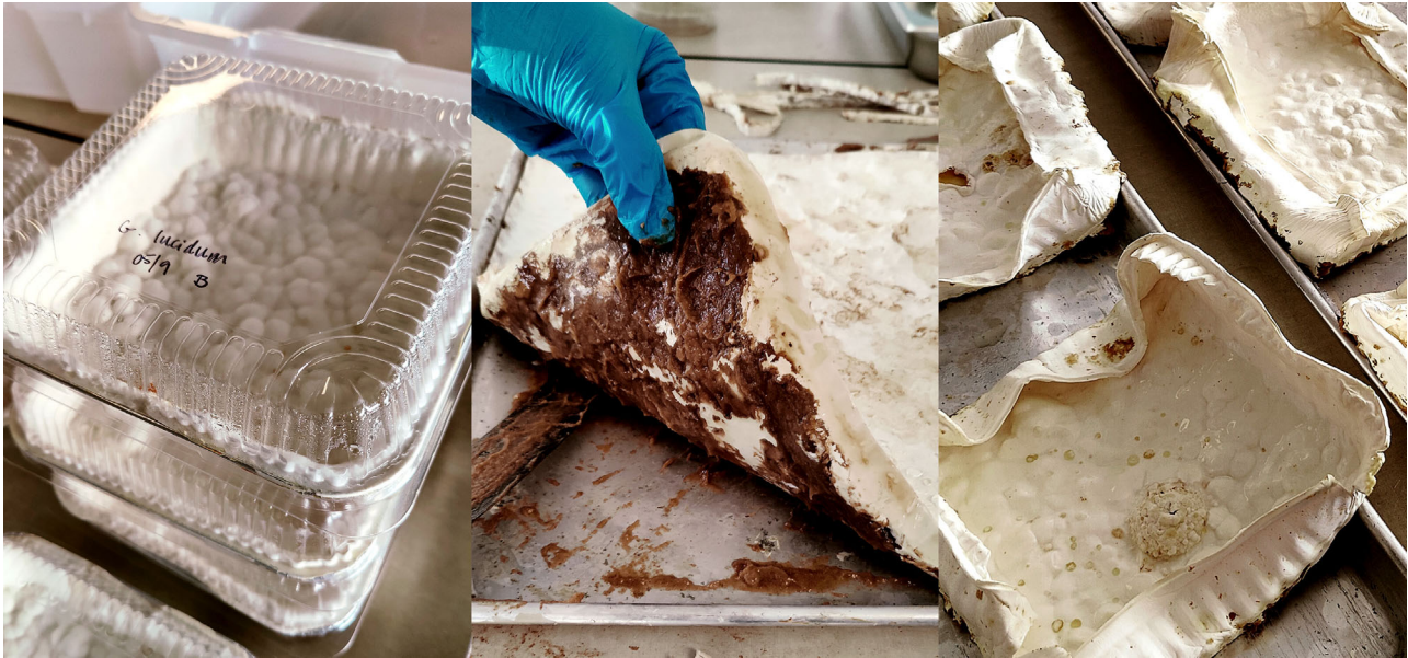
Figure 1. (Left) Ganoderma lucidum (rishi) grown in aluminum trays with clear plastic lids, (Middle) Large mat of Ganoderma lucidum (rishi) being harvested via peeling, (Right) Mycelium mat after harvesting and rinsing of growth media residue.
