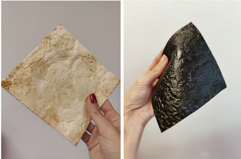
Figure 10. (Left) Mycelium leather grown using agar culture on paste, treated with 10% glycerol for 72 hours and heat-pressed, (Right) Same treatment with black leather dye.
