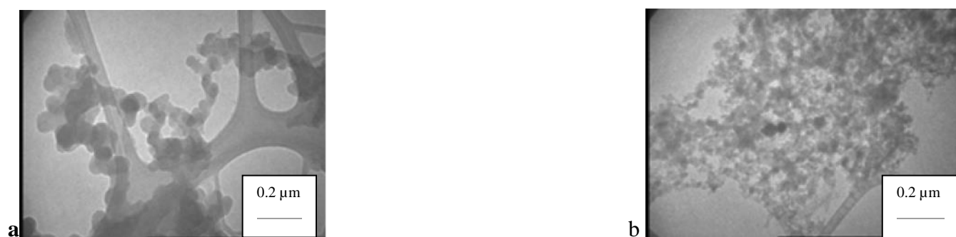
Figure 1. Organic conglomerates in a) Chain and in b) Mass obtained by TEM
