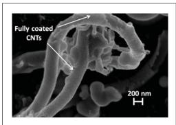
Scanning electron micrograph of multiwalled carbon nanotubes coated with BaTiO<sub>3</sub>.
