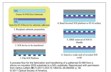
to transfer electronic and photonic devices without compromising structural integrity and functionality.
