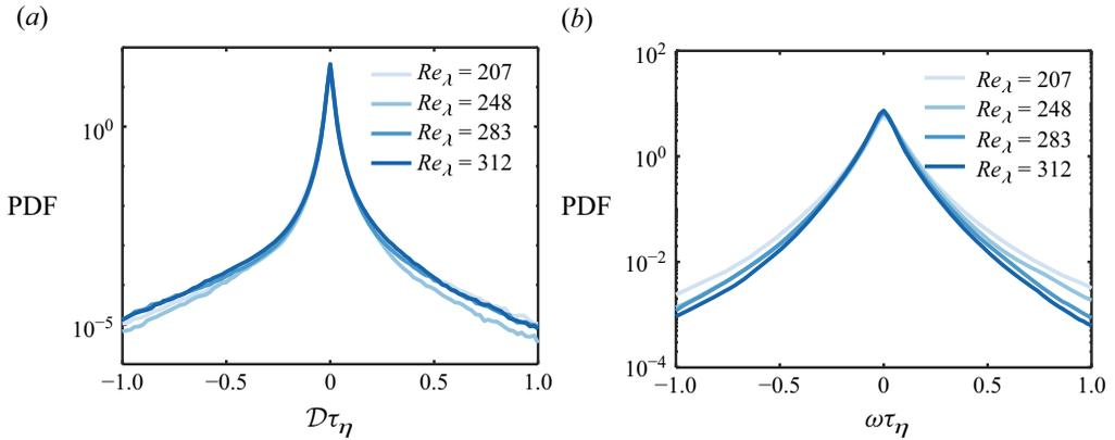
Figure 4. The PDFs of surface divergence  $\mathcal{D}$  (panel (a)) and vorticity  $\omega$  (panel (b)) at various  $Re_\lambda$ . In both panels, darker colour represents higher  $Re_\lambda$  and vice versa.
