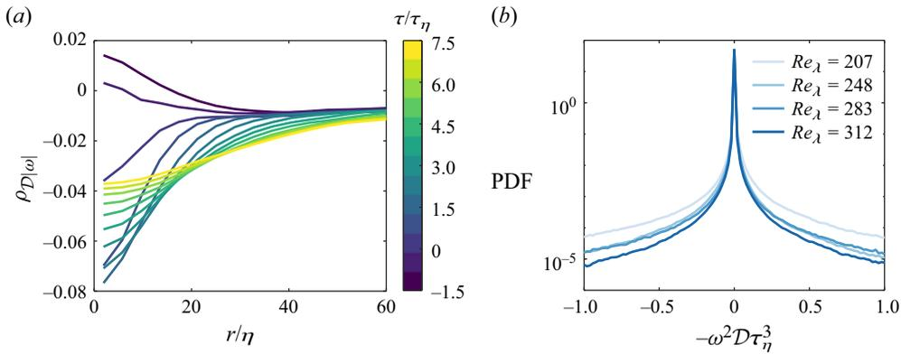
Figure 14. (a) The spatial-temporal cross-correlation between the divergence and vorticity magnitude as a function of separation distance. The colours represent the time delay  $\tau$ . (b) The PDFs of the vortex-stretching term. The darker colour represent the higher  $Re_\lambda$ .
