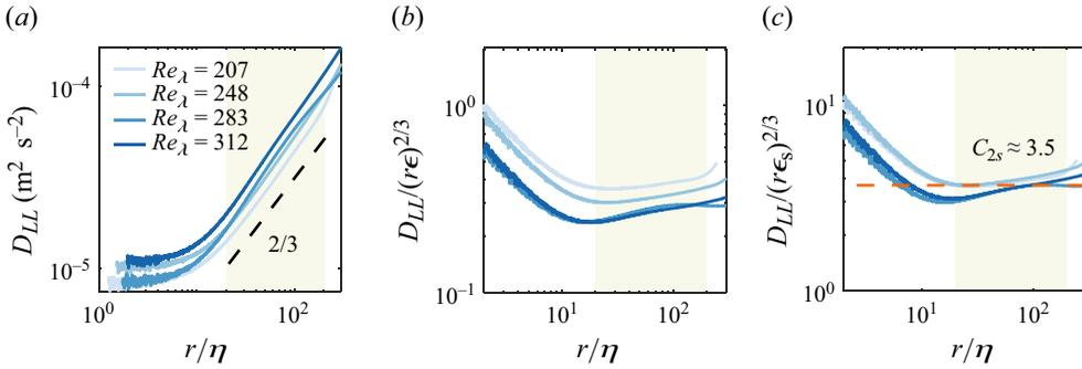
Figure 9. (a) The longitudinal second-order structure function  $D_{LL}$  as a function of the separation distance. The dashed line denotes  $2/3$  power-law scaling. (b) Value of  $D_{LL}$  normalised by  $(r\epsilon)^{2/3}$ . (c) Value of  $D_{LL}$  normalised by  $(r\epsilon_s)^{2/3}$ . The orange dashed line marks  $C_{2s} \approx 3.5$ . In all of the panels, the darker colour represents high  $Re_\lambda$  and *vice versa*. The green shaded area marks the inertial range.
