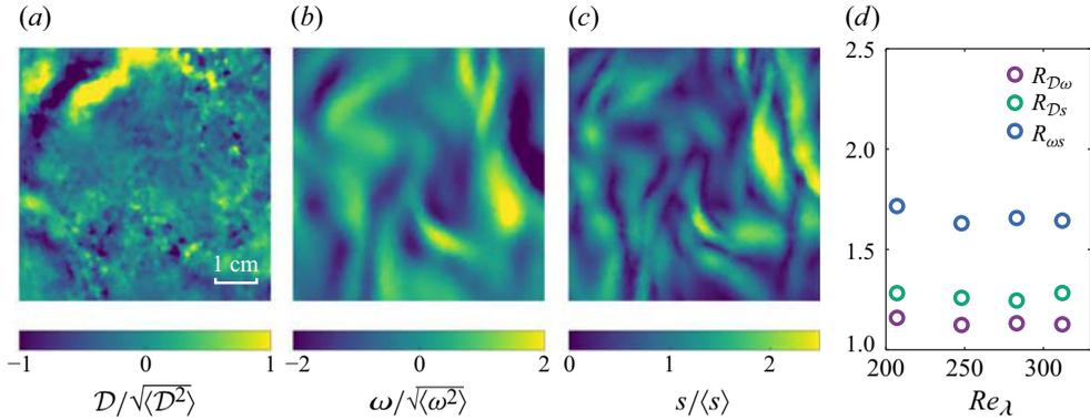
Figure 8. (a–c) Snapshots of surface divergence field (a), vorticity field (b) and strain field (c) on the free surface  $Re_\lambda = 312$ . (d) Overlap coefficients as a function of  $Re_\lambda$ . The purple, green and blue symbols represent divergence–vorticity, divergence–strain and vorticity–strain overlap, respectively.
