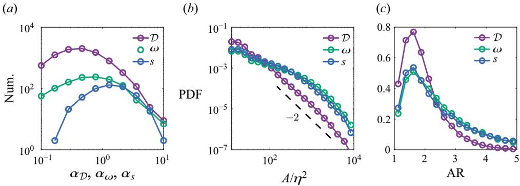
Figure 7. (a) The number of high-intensity objects found in the FOV as a function of thresholds. (b) The PDFs of the normalised area of high-intensity objects. The dashed line marks the power-law scaling of  $-2$ . (c) The PDFs of the aspect ratio of high-intensity events. In all of the panels, the purple, green and blue symbols represent high-divergence, high-vorticity and high-strain objects, respectively. Only the data for  $Re_\lambda = 312$  are included.
