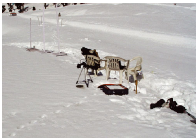
Fig. 2. Field set-up of ASD spectroradiometer for soil contamination experiment.
