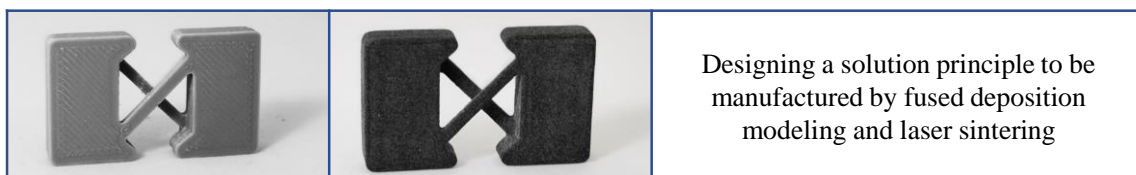
Figure 3. Solution principles to channel energy manufactured by fused deposition modeling with polylactide (left) and laser sintering with PA12 (center)
