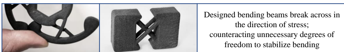
Figure 6. Solution principle with double bending beams (manufactured by laser sintering)
