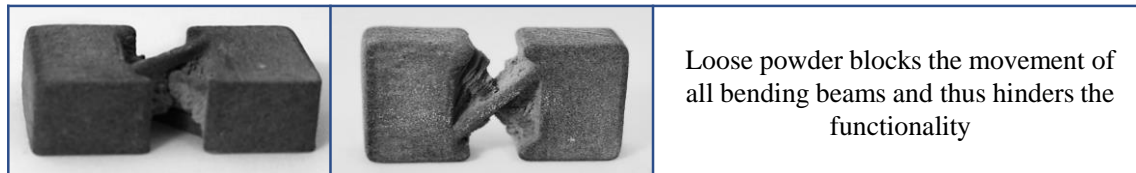
Figure 9. Solution principles with necessary post-processing after laser sintering
