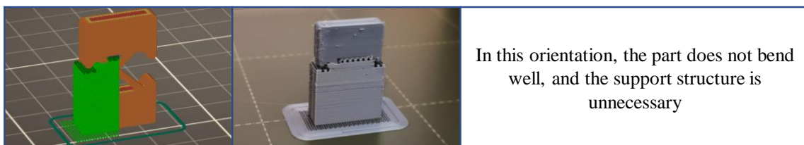
Figure 5. Negative example for part orientation of a solution principle (manufactured by fused deposition modeling)
