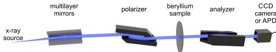
Figure 13. Sketch of the experimental setup investigating CRL material properties. The multilayer mirrors collimate the X-rays from the rotating anode X-ray source. The combination of the polarizer, analyzer and charge-coupled device camera allows for polarization sensitive imaging. Reprinted from Ref. [61], with the permission of AIP Publishing.
